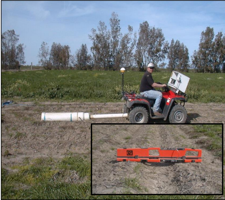
Fig. 2. Two EM instruments are housed inside a PVC casing and towed behind an ATV with GPS system. The inset shows the orientation of the two instruments inside the PVC housing. One is horizontal (shallow) and the other is vertical (deep) mode.
